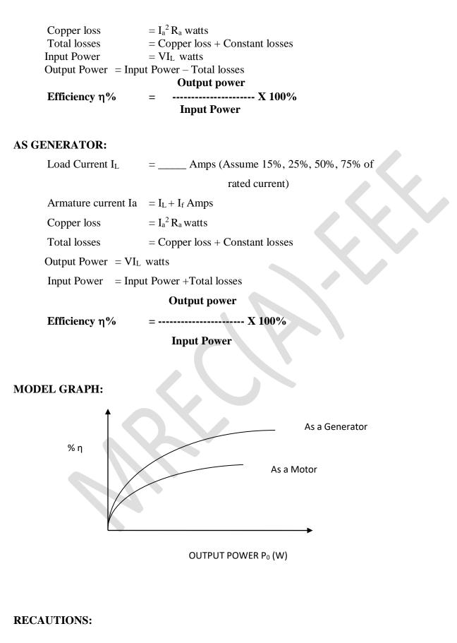
1. The field rheostat should be in the minimum position at the time of starting and stopping the motor DEPARTMENT OF ELECTRICAL AND ELECTRONICS ENGINEERING
